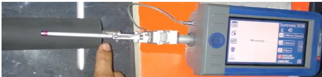
FIG. 1 Preparing the test sample for testing the Surface Roughness
