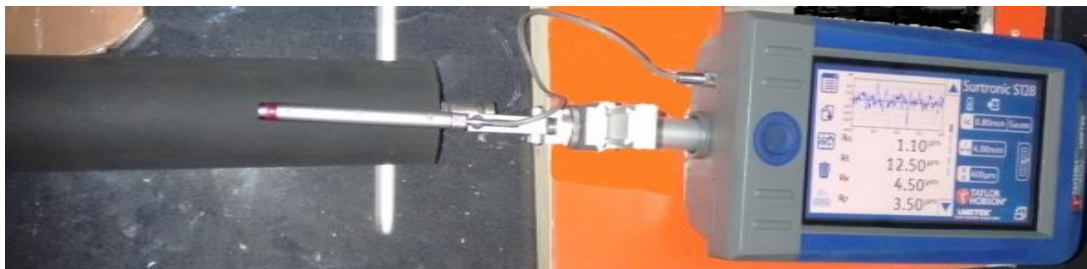
FIG. 2 Test result of the Surface Roughness
